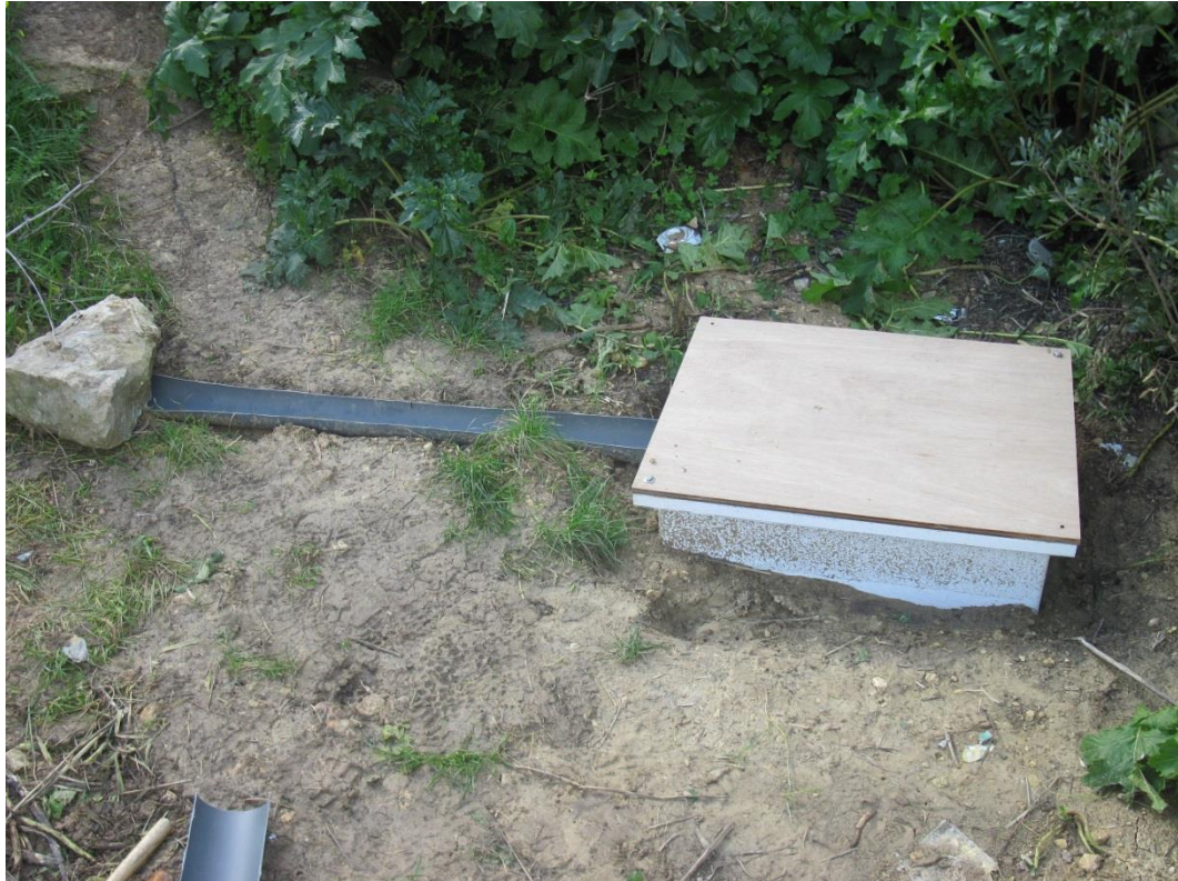
Figure 2: The gutter for Silt Trap 2 as it was before it was moved to a better position to improve the flow of water. With the previous position water was found to be diverted away from the gutter resulting in a reduction of water entering the silt trap.
